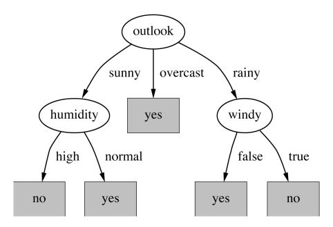
Note: not all leaves need to be pure; sometimes identical instances have different classes ⇒ Splitting stops when data can't be split any further
